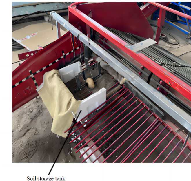
Figure 4. Potato friction test process performed in the experiment
