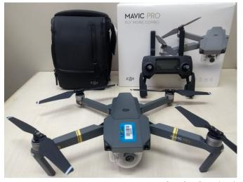
**Figure 1.** Dà-Jiāng Innovations Science and Technology (DJI) Mavic Pro quadcopter Remotely Piloted Aircraft System (RPAS)
