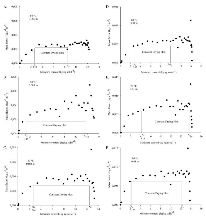
**Figure 1.** Experimental data of mass flux as a function of moisture content during convective drying of crushed jambu leaf paste at temperature 60 °C and thickness 0.005 m (A), temperature 70 °C and thickness 0.005 m (B), temperature 80 °C and thickness 0.005 m (C), temperature 60 °C and thickness 0.01 m (D), temperature 70 °C and thickness 0.01 m (E), and temperature 80 °C and thickness 0.01 m (F)
