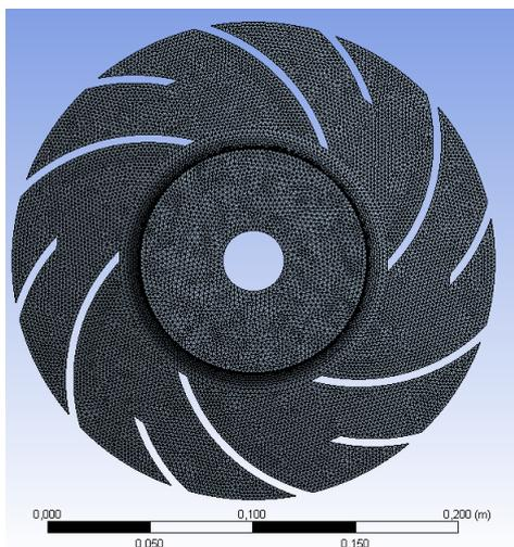
**Figure 2.** Mesh generated with six splitter blades at outlet (impeller#2)
