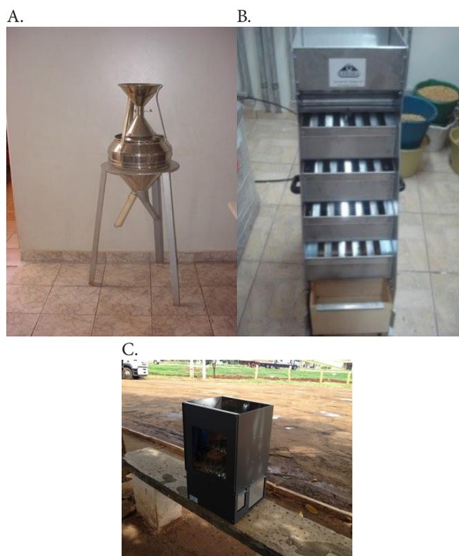
**Figure 1.** Illustration of the devices evaluated for homogenization and dilution of samples: Boerner (A); 16:1 multichannel splitter (B) and 4:1 multichannel splitter (C)
