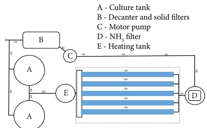
Figure 1. Aquaponic system operation scheme
