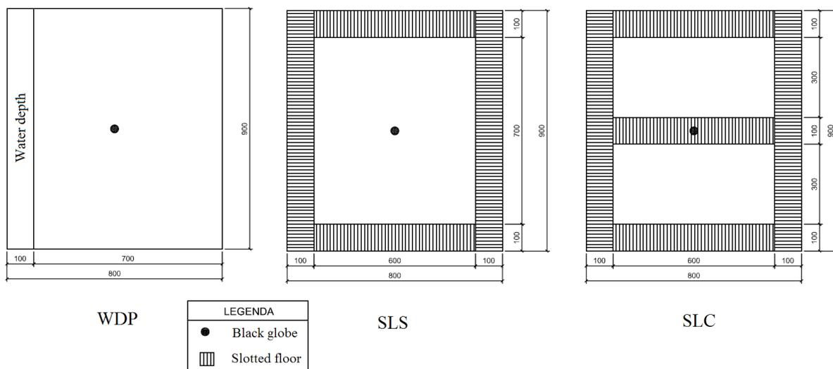
Figure 1. Floor plan of the pens (WDP: Water depth, SLS: slotted floor on the sides and SLC: slotted floor in the center and sides)
