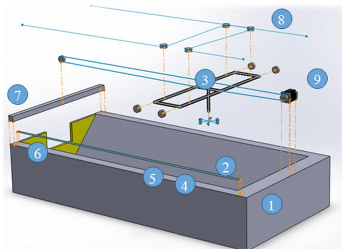
1) Open channel; 2) Rail; 3) DAM; 4, 5 and 6) Reed switches; 7) Pulley support; 8) Orthogonality system; 9) Traction system
