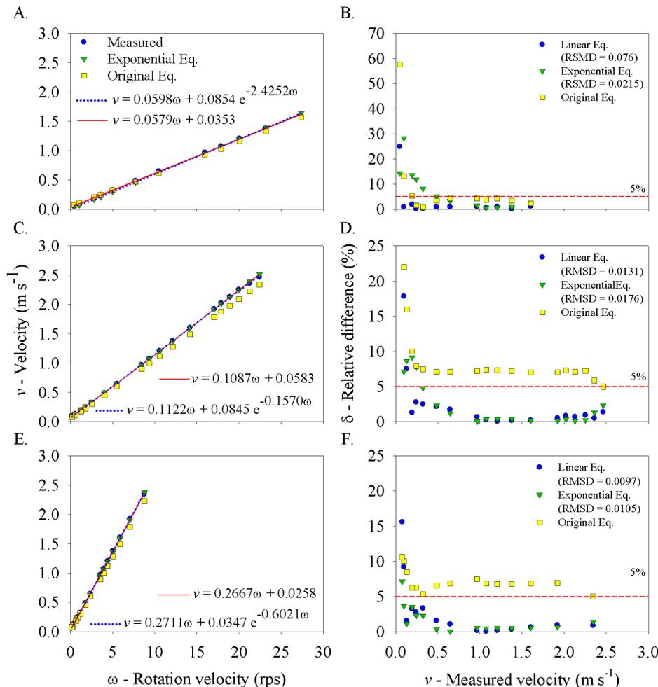
Figure 4. Equations for the Miniature current meter and the respective relative differences,  $\delta$ : (A) and (B) - propeller 1, (C) and (D) - propeller 2 and (E) and (F) - propeller 3
