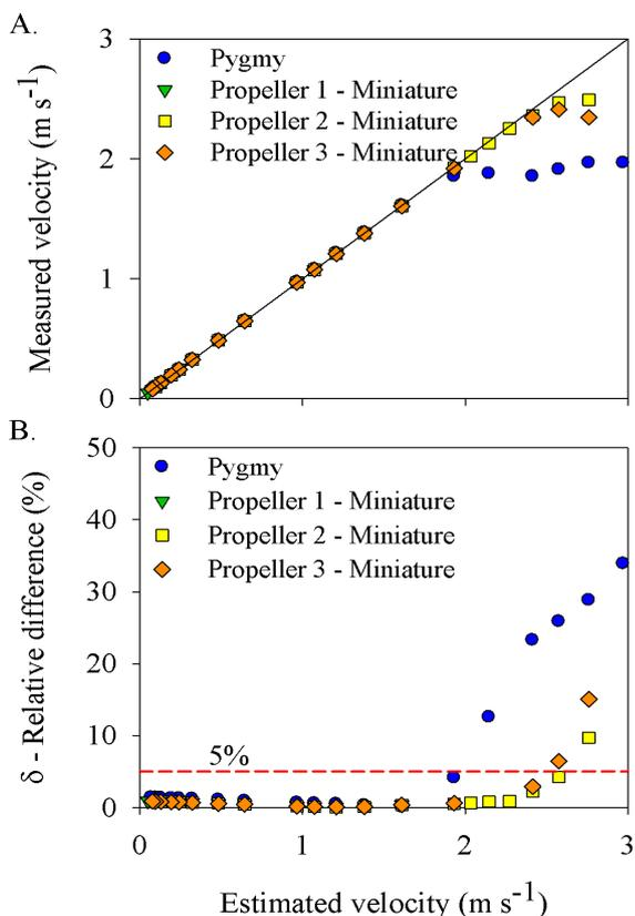
Figure 2. Relationship between estimated and measured velocities (A) and relative difference for the measured velocities (B)
