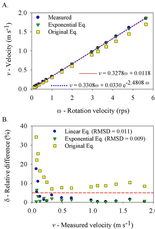
Figure 3. (A) Equations of the Pygmy current meter and (B) Relative differences,  $\delta$
