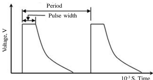
**Figure 1.** Pulse format produced by the controlled pulse generator
